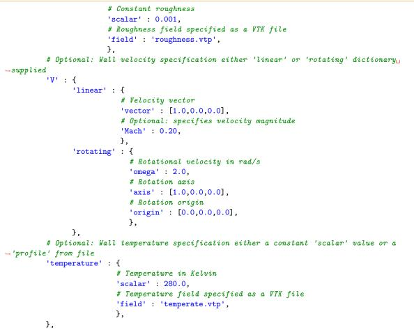
**Note:** The roughness at each boundary face is set by finding the nearest point to the face centre on the supplied VTK file with the roughness value looked up in a node based scalar array called 'Roughness'
