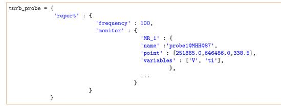
The '*frequency*' is the number of solver cycles between outputs, and the '*monitor*' defines the name of the probe using the WindFarmer standard notation.
